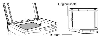
Gently close the original cover. When copying a book or an original which has been folded or a crumpled original, press down the original cover lightly. If the original cover is not securely closed, the copies may be striped or blurred.
